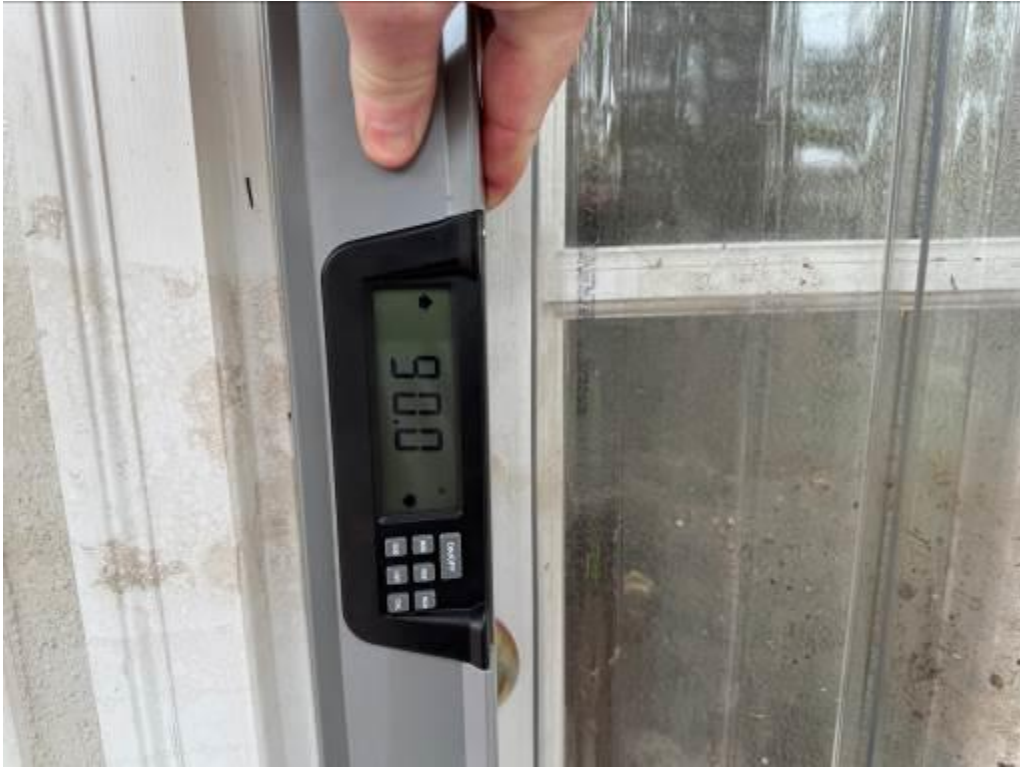
Photo No. 11: No listing/leaning observed to structure (typical).
